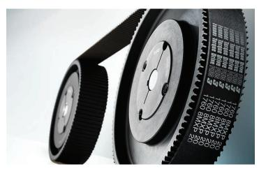
Synchronous belt drives operate by positive meshing and do not require high installed belt tensions. For optimum performance, however, belts should be installed with a pre-tension suitable for the envisaged drive duty, derived from the
